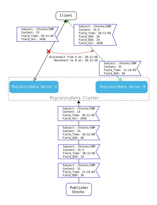
Figure 5.7: Example of Data Recovery With Guaranteed Message Delivery Enabled
