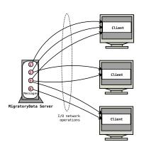
Figure 5.4: Circulation of Messages without Batching
